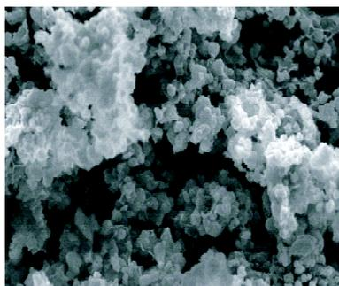
**Fig. 2** SEM micrographs of porous hydroxyapatite/chitosan composite(SEM, × 4.00K)
